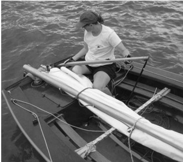
Sarah Pedersen adjusts the tiller bar on W8705. Nick and Chip fashioned a “Butt Bar” across the rear seats of the boat so Sarah could slide back and forth as she tacked.
