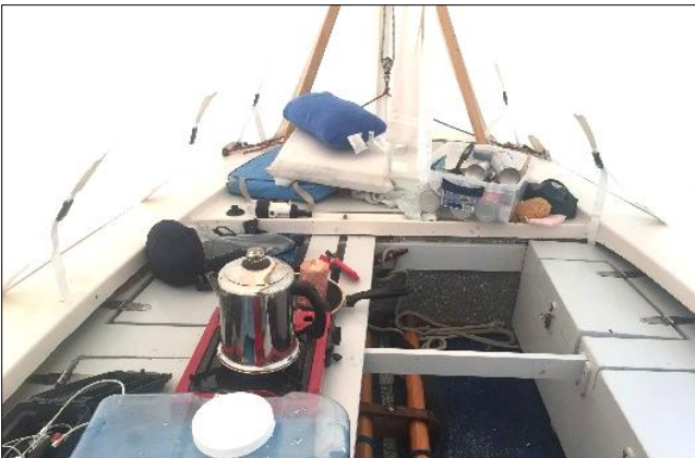
Dan Roeder has customized his Wayfarer cockpit to include lockers and a sleep platform.
