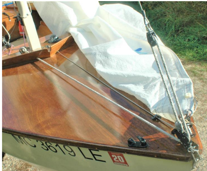
This is Solje 's Hirsch forestay gun block arrangement. The jam cleat is next to the mast beyond the splashboard.
